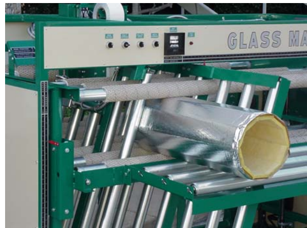
Closing 10-sided, “round” duct with the versatile DC-36 Close Master for smooth, sure tape sealing.
